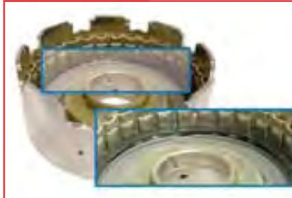
DrumSavers™ prevent the replacement of expensive drums. By installing Alto components further damage to the existing drum will be prevented, allowing the drum to perform as designed.
