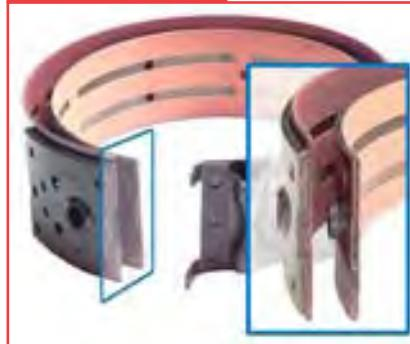
PowerBands® enhance torque load and improve shift quality. They are designed wider than the original band to increase stopping capacity of up to 25%. Anchors have been increased in thickness and heat treated when required to eliminate premature failures.
