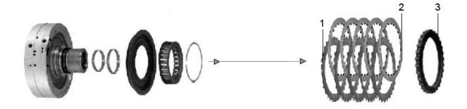
**Installation:** Stack the Intermediate clutch pack as follows; install .461" stepped pressure plate (3) into case, step side down, install .076" friction plates (2), install .077" Kolene® steel plates (1) into case, You will be alternating friction and steel plates, 5 friction plates and 5 steel plates, ending with a steel plate, install piston, return spring, and snap ring into center support, install center support into case.
